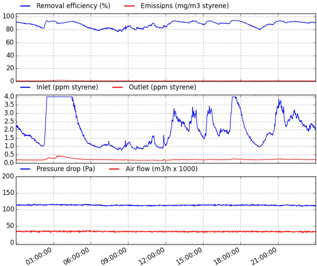
Figure 5: Summary of data from a CLIMATIC installation during one day of normal production of a major European blade OEM. As can be seen, the emissions are constantly very low, and the removal rates are very high.
