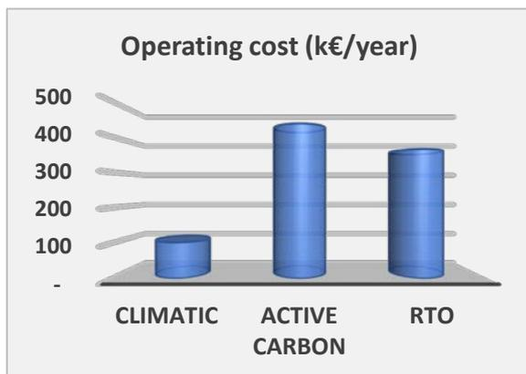
Figure 1: Examples of operating cost of a single emission point on a wind turbine blade production line of 50,000 m<sup>3</sup>/h (see section 6 for further information).
